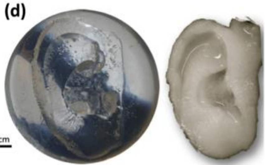
d) Negative silicone mold used to guide the bacteria during the bacterial culture to reproduce the large-scale features of the outer ear (left) and 3D BC implant prototype (1% BC) produced in the shape of the whole outer ear according to the 3T MRI scanning technique (right)
